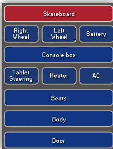
Figure 10 Installation order chart
