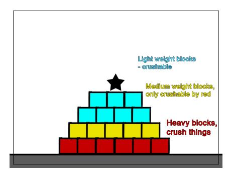
**Summary of the principle** - Heavier weights lower the center of mass, keeping the objects stabilized on the ground
